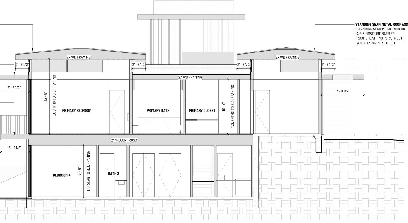
STANDING SEAM METAL ROOF ASSEMBLY -STANDING SEAM METAL ROOFING -AIR & MOSITURE BARRIER -ROOF SHEATHING PER STRUCT. -WD FRAMING PER STRUCT
